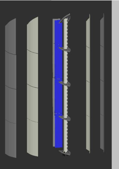
The CAD drawing to the left was Signature's shop drawing. We wanted to show them that we were going to add a layer of acrylic to help keep the bugs out of the fixtures. We also wanted to change the glass on the back to acrylic so it would be harder and less dangerous if the back panel broke. These CAD drawings help show the designers what we want create and the also help the contractor understand how to install the fixtures.
