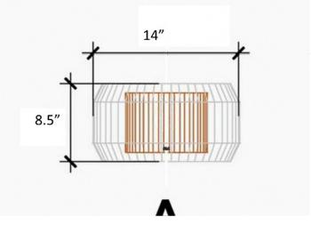
14" diameter acrylic clear shade shade 10" amber shade 14" mold from two halves. Halves are joined and seam is finished with metallic strip. 10" diameter amber acrylic shade rolled and seamed vertically at one joint. For single unit pendent the unit is held by two cable to canopy. Used GU24 Base Socket, does not include lamps.
